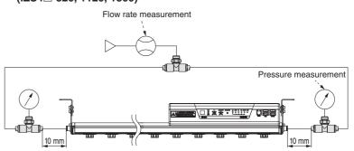
c) Double sided air supply (Connecting tube: O.D. Ø8 x I.D. Ø5) (IZS4□-1600, 1900, 2320, 2500)
